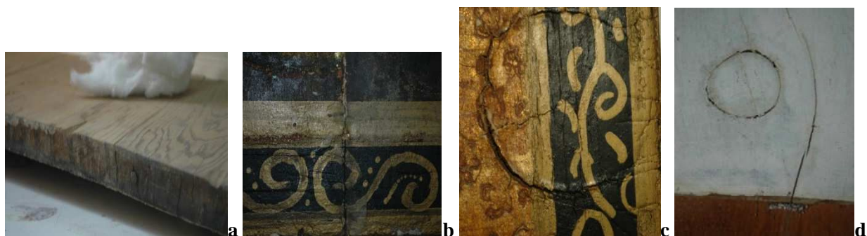
Fig. 7. Images showing bending, curving (a) cracking of the icon (b) and the separation of large-sized wooden knots (c, d).
