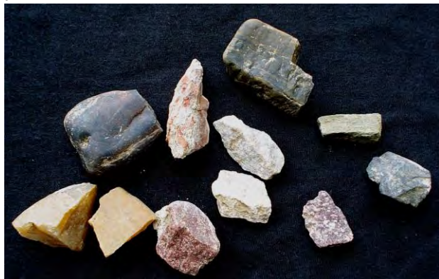
Fig. 27. a. Fragment of the northern wall of the portico cloister (Photo by F. Mărginean); b. Scrap tesserae of river stone, red marble, and red porphyry collected from the embleton of the northern wall of the portico.
