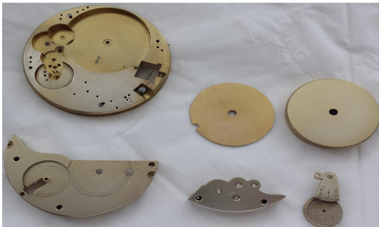
15. movement parts after cleaning
