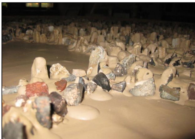
11 a, b. The aspect of the surface after the first layer of fine roman cement was casted
