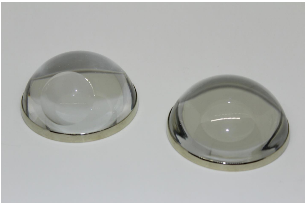
8. half spheres casted, finished, beveled and mounted into the metal frames
