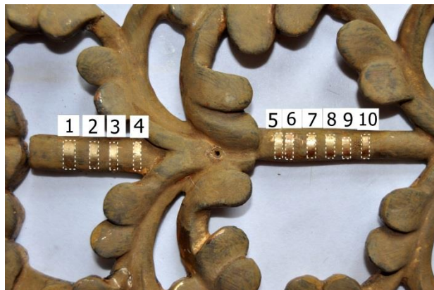
5. Tests for removing the primer from original gold
