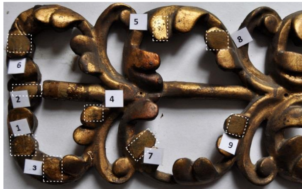
4. Tests for removing the imitation of gold and linseed oil glue
