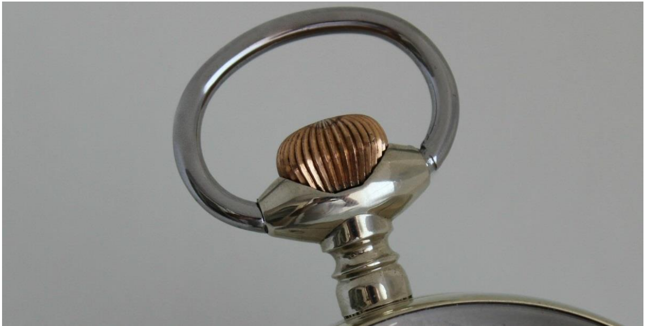
7. new lathe made pendant ring
