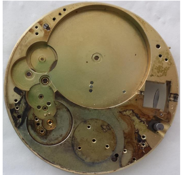
4. movement plate view, before restoration
