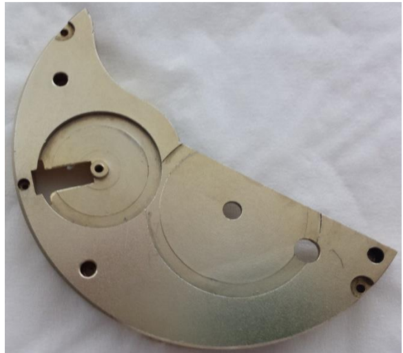
14. barrel bridge after cleaning
