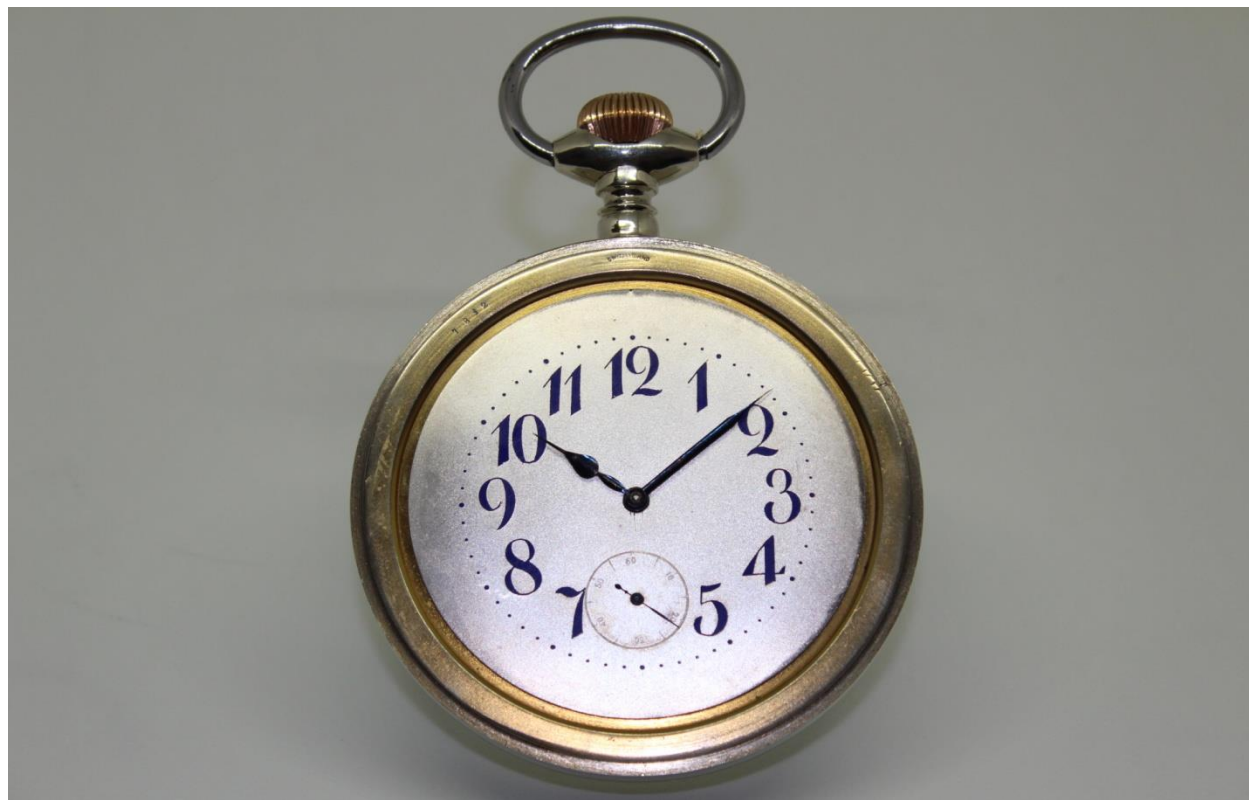
20. dial view after mounting into case, without crystal
