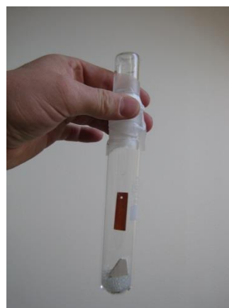
3. Measurement of carboxylic acids by passive samplers in a display case. From a Danish museum. 4. Glass test tube with a material sample and a metal coupon, ready for the accelerated corrosion test (‘‘Oddy test’’).
