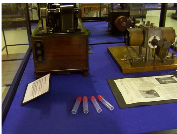
3. Measurement of carboxylic acids by passive samplers in a display case. From a Danish museum. 4. Glass test tube with a material sample and a metal coupon, ready for the accelerated corrosion test (‘‘Oddy test’’).
