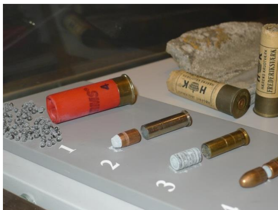
1. Corroded museum objects. Exhibition of gun bullets with white powdery lead corrosion due to corrosive vapours given off by the display case. From a Danish museum.
