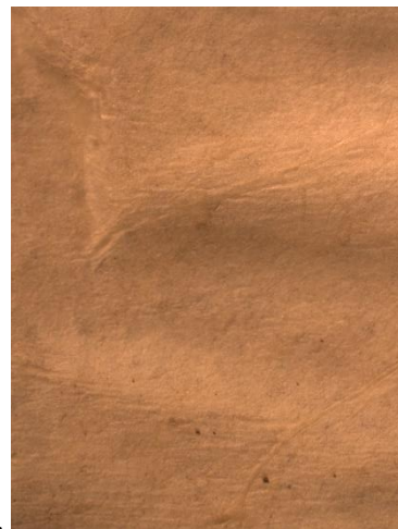
39. Page 40 surface detail, loss of flatness middle right edge, photomicrograph 20x
