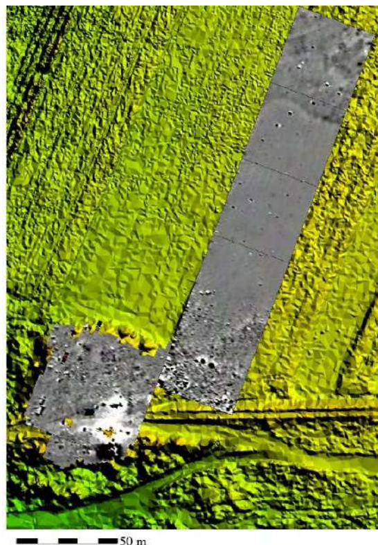
Fig. 4 – The results of the geomagnetic investigation superimposed on the digital terrain model
