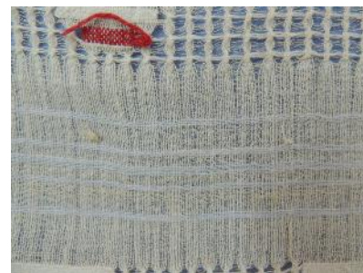
Fig. 9. Defect de țesere - fire innodate.
