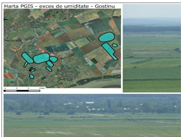
Figure 2. Gostinu PGIS Map and pictures showing effects of water infiltration through the levee
