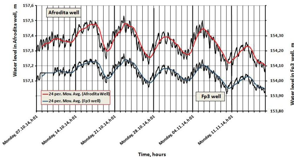
**Figure 8.** Weekly fluctuations of the thermal aquifer level measured in Afrodisita and Fp3 wells.
