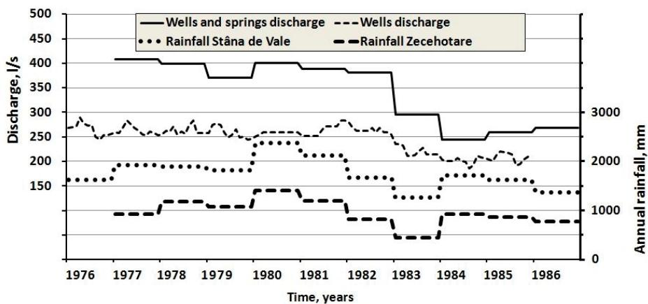
**Figure 3.** Evolution of the flowing potential of the thermal aquifer based on Cohut & Paal (1985), together with the annual amounts of precipitations at Zecehotare and Stâna de Vale between 1976-1986.
