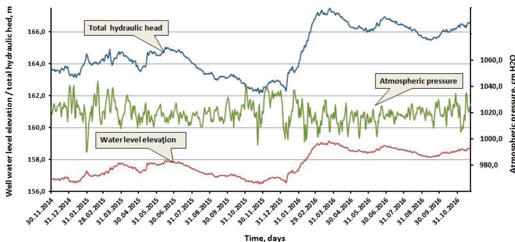
**Figure 6.** The total and measured heads in Afrodită well and atmospheric pressure at station 1 Mai for november 2014 to november 2016 time period.
