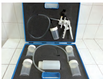
Figure 5. Kit for water sample collection equipped with suction-lift pump.
