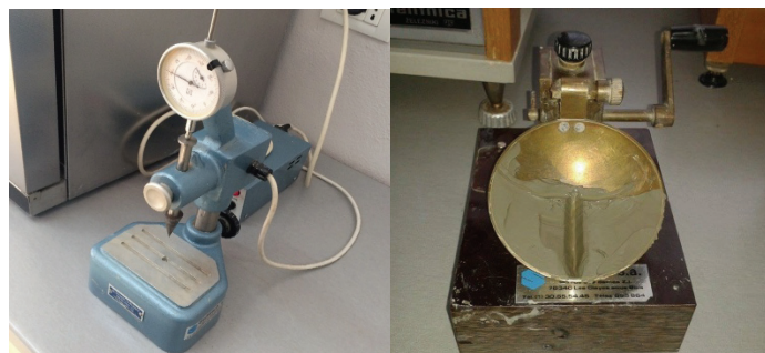
Figure 2. Casagrande and Fall-cone test apparatuses (original).
