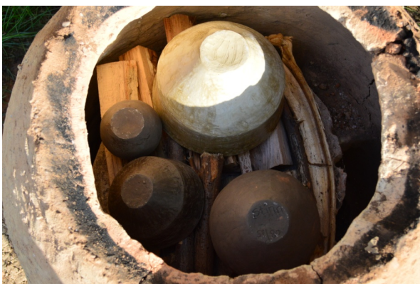
Figure 5. Placing the dried pots bottom-up on the layer of combustion.
