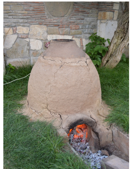
Figure 6. The kiln during firing (640°C).
