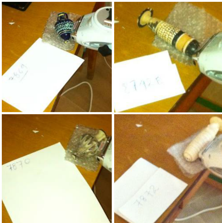
Figure 1. Images of the glass vessels from Delphi, during the in situ XRF analysis
