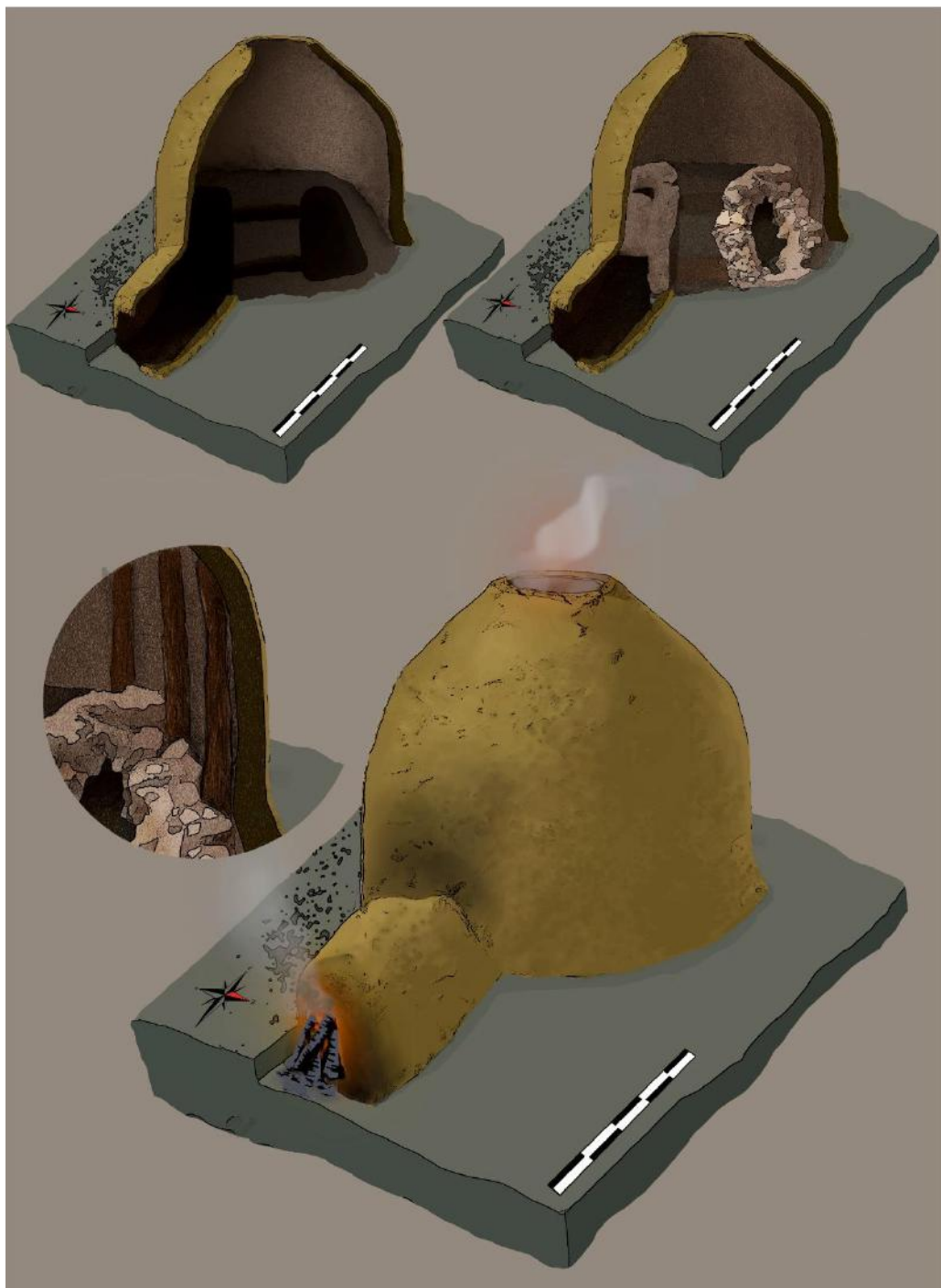
Figure 11. Graphic reconstruction proposal of the pottery kiln from Cucuteni-Cetățuie and its manner of use (drawings by B.Ș. Novac).
