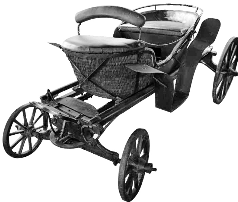
Fig. 13. Tarantas on an iron undercarriage, with wings over the wheels and sprung suspension
