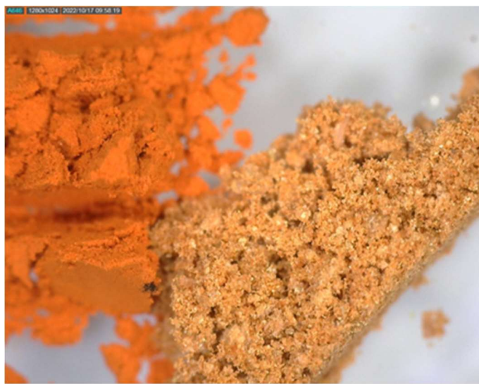
Fig. 25. Red iron oxide: left side – synthetic; right side – mineral oxide from local sources
