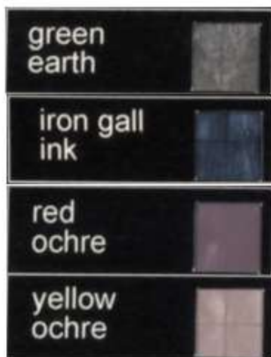
Fig. 26. Technical photography images of the experimental icon in the visible light range (VIS) and the corresponding one with a polarized filter (POL) and halogen lamps (2 x 400W). Images of the green earth, red ochre, yellow ochre and iron gall ink from the pigment checker (POL) were used for comparison and for checking the areas where each of these pigments, also identified by XRF, were employed for painting the icon
