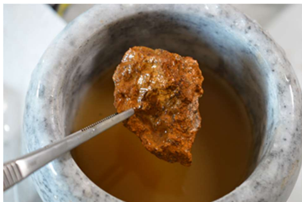
Fig. 17. Iron-bearing water – the source of bog iron formation. Bog iron found in Rachiş Valley
