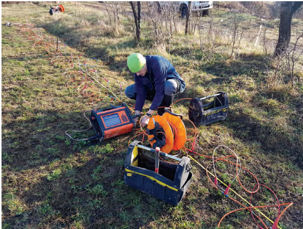
Fig. 6 – Electrical Resistivity Tomography measurements in the area of eastern gate, Pojejena (2019). Radoslaw Mieszkowski setting the instrument.
