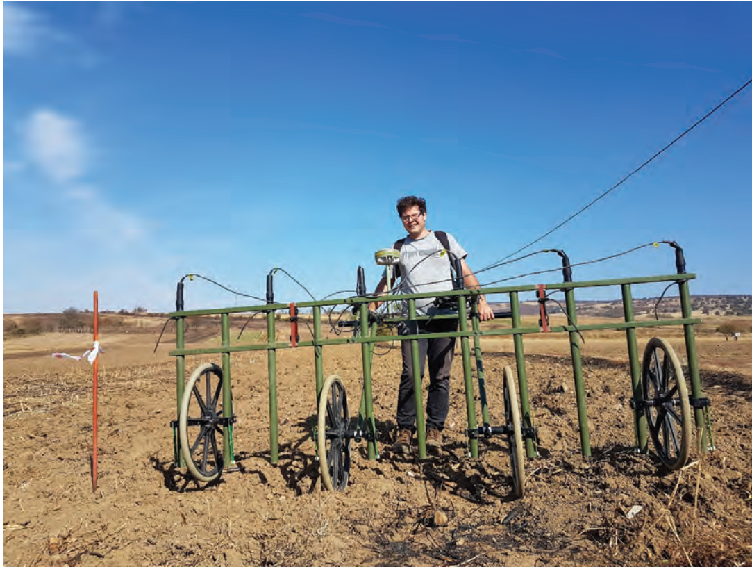
Fig. 5 – Magnetometry survey in Pojejena (2018) with the use of multi-channel SENSYS MX V3 magnetometer. Wiktor Rutkowski behind the bar.
