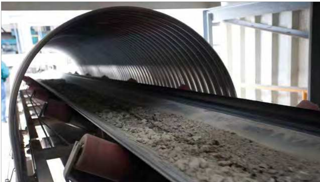
Dry slag conveyor belt, buffer bunker feed
