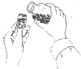
FIGURE B-19 Removal of a solid from a glass-stoppered bottle.
