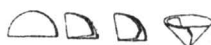
F-9 Alternative method of folding filter paper. Steps in folding filter paper for use in filtering with a regular funnel. The second fold is not exactly at a right angle. Note tear.
