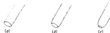
B-5 (a) After cut. (b) After fire polishing. (c) The end has been heated too long.
