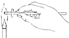
B-4 Fire polishing (note rotation of the work).
