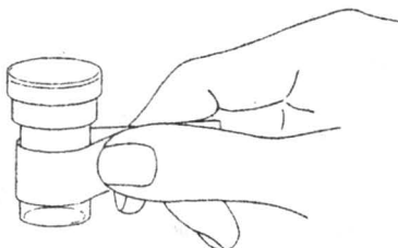
FIGURE K-4 Weighing bottle and method of handling it.
