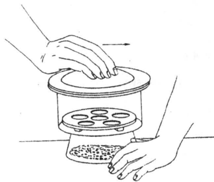
K-7 Removing desiccator cover.
