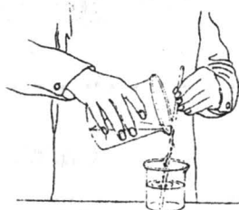
B-23 Use of stirring rod to guide liquid.
