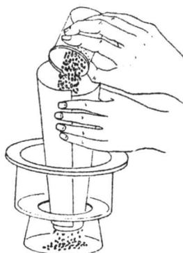
FIGURE K-8 Filling desiccator with fresh desiccant.
