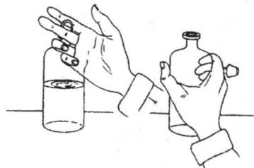
B-21 Handling a glass stopper.
