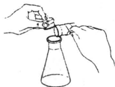
FIGURE K-5 The weighing operation.
