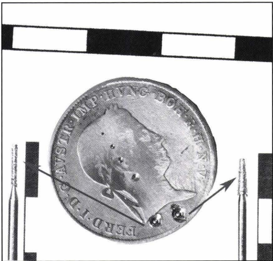
Fig. 4 – The picture of coin no. 6 after drilling with two types of cylindrical cutters. On the picture the holes after drilling are shown.
