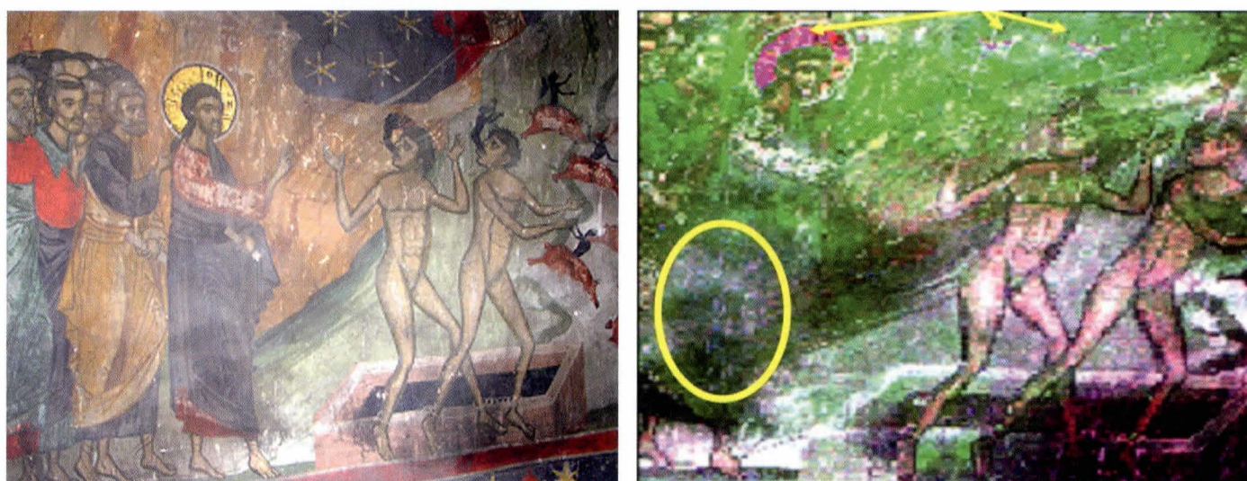
Fig. 4 – Picture of the fresco “Jesus Heals the Demon-Possessed of Gadarenes” (Matthew 8, 28-33) in Sucevita (top). The corresponding false color image (bottom), obtained with the scanning LIF system operating at 266 nm, highlights in dark blue the presence of fungi on the lower part of Christ's dress (circled), conversely the red color of the gilding on the aureole and stars (marked by arrows) does not permit to discriminate the use of paraloid during the restoration.
