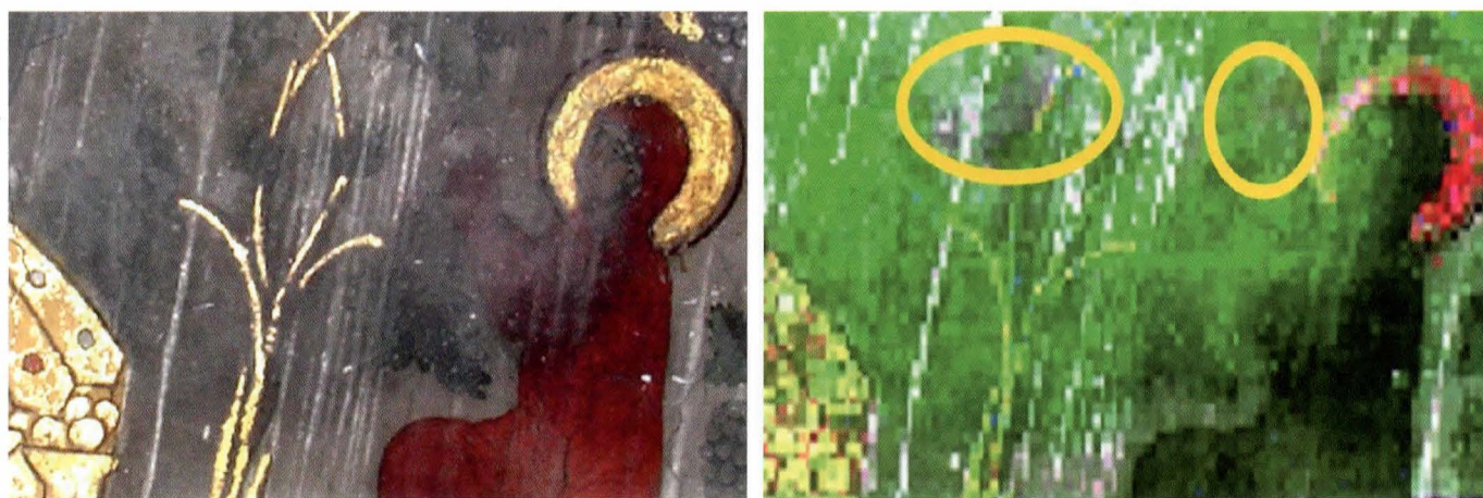
Fig. 5 – Picture of the Saint at Christ’s right side in “Christ King” fresco in Sucevita (top). The corresponding false color image (bottom), obtained with the scanning LIF system emitting at 355 nm, highlights: in green, the pigments; in white, pigments discoloration; in red, the gilding; in purple, fungi (main areas of biological attack circled by a yellow line).
