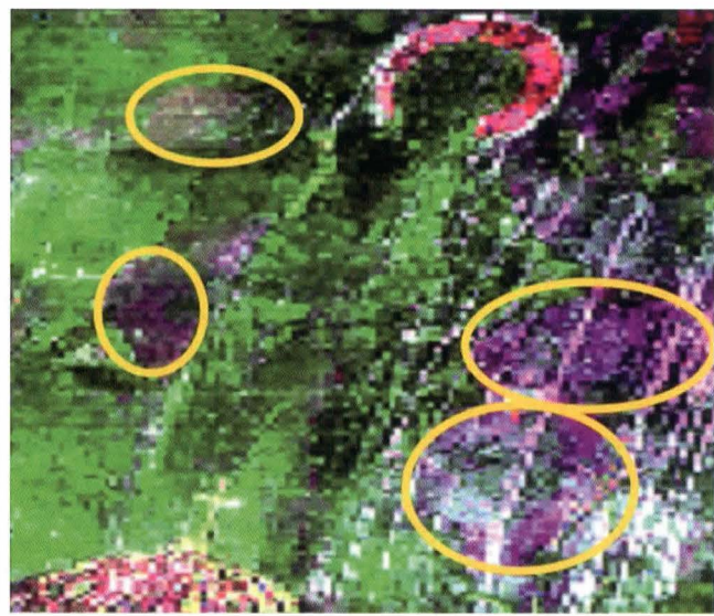
Fig. 6 – Picture of Christ in “Christ King” fresco in Sucevita (left). The corresponding false color image (right), obtained with the scanning LIF system emitting at 355 nm, highlights: in green, the pigments; in white, pigments discoloration; in red, the gilding; in purple, fungi (main areas of biological attack circled by a yellow line).
