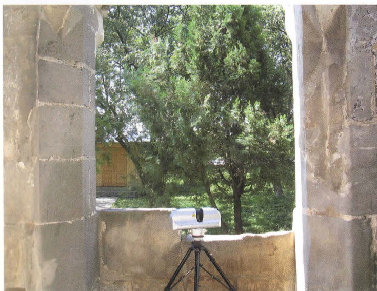
Fig 2.4 Scanning the interior of the porch
