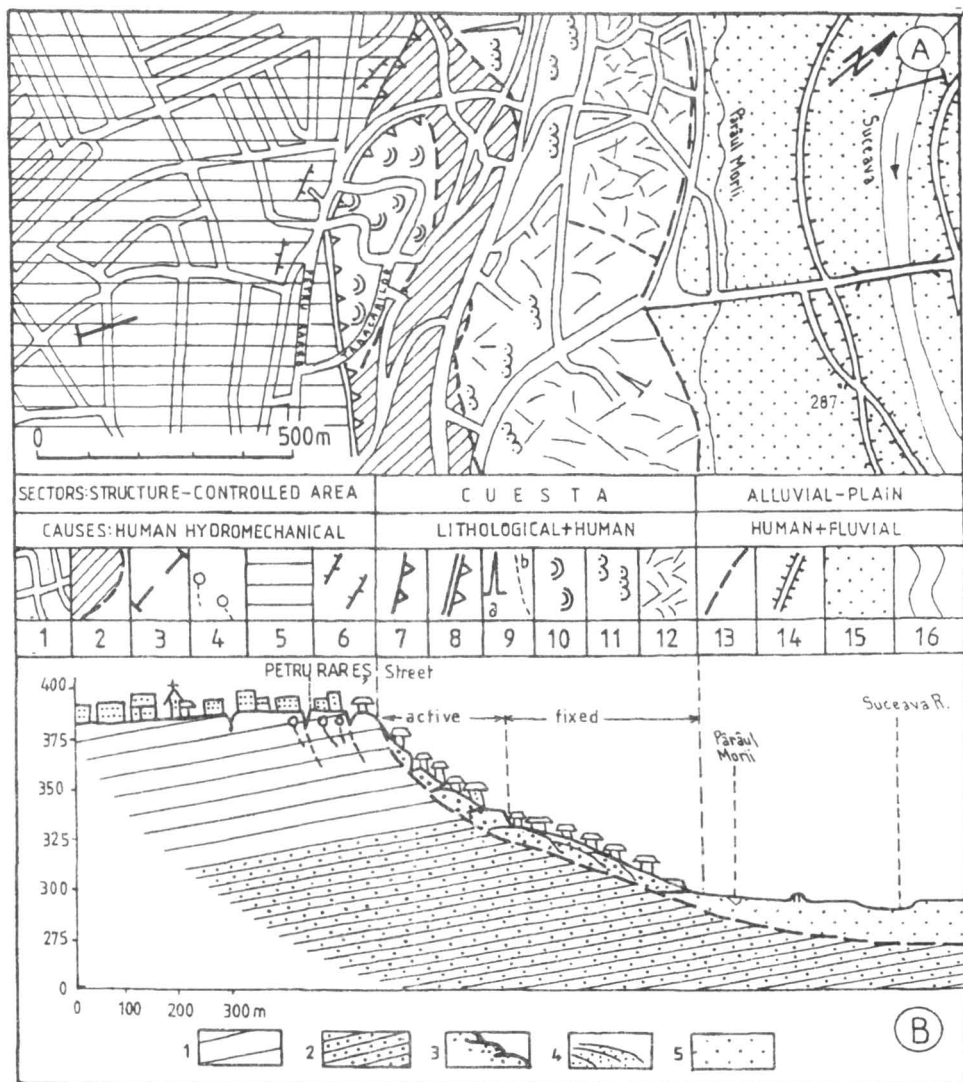
Fig. 5 – Succava landslide: A , Geomorphological map. 1, Street network; 2, older landslide-affected area; 3, profile line; 4, water source from the city's sewerage system; 5, structure-controlled surface; 6, recent creeks; 7, cuesta cornice; 8, active scar; 9, gullies (a), ravines (b); 10, active slides; 11, sliding deluvia; 12, sliding glacia; 13, glacia line toward the floodplain; 14, dams; 15, floodplain; 16, secondary channel. B , Slide profile: 1, sands with clay and sandstone intercalations; 2, Burdujeni oolitic sandstone; 3, mobile brittle formations; 4, old sliding deluvium; 5, alluvial deposits.
