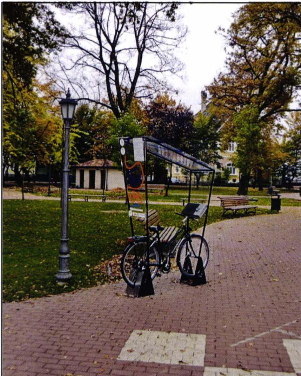
**Fig. 7. Bike charger for electronic devices (phones, tablets) in the Central Park**
