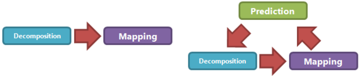
FIG. 1.1. Interaction between components of a Parallel Scheduler; arrows indicate how components influence each others: (left) Traditional approach; (right) Our system with the Predictor.
