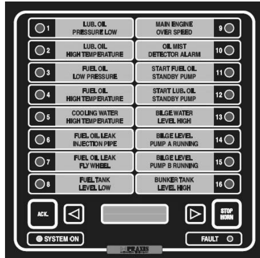
b) Alarm Panel of MINI-GUARD
